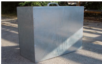
Sound insulation hood for the power unit
