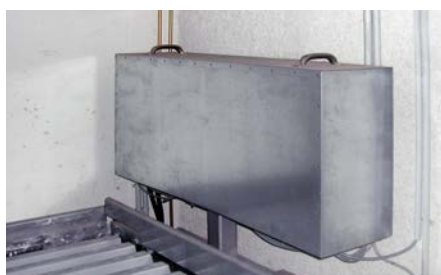
Sound insulation hood for the power unit
