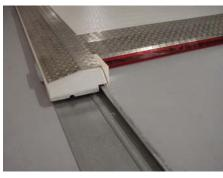
Extra sheet is placed next to the chain guide. It is a protection against sediment (result of the circulating transport chain)
